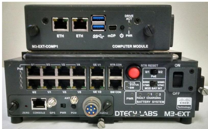
Figure 5: DTECH Example M3-EXT VPN Remote Node
