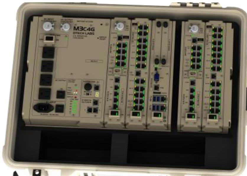
**Figure 3: DTECH M3C4G Products in a Hard Sided Case**
